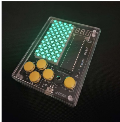
Figure 2. Completed game machine with the LED matrix illuminated.
